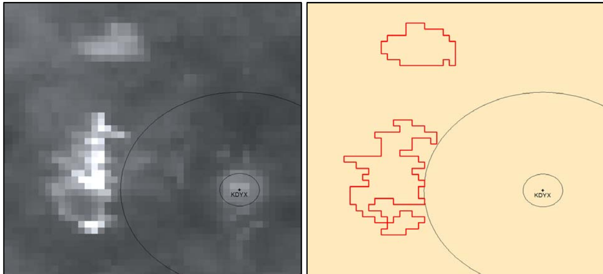
Figure 3: Left Image - 12-month Q2 QPE showing bright “hot spots” west of Dyess AFB, TX WSR-88D (KDXY) with 3- and 18-km range rings. Right Image - NSSL-generated polygons outlining QPE “hot spots.”
