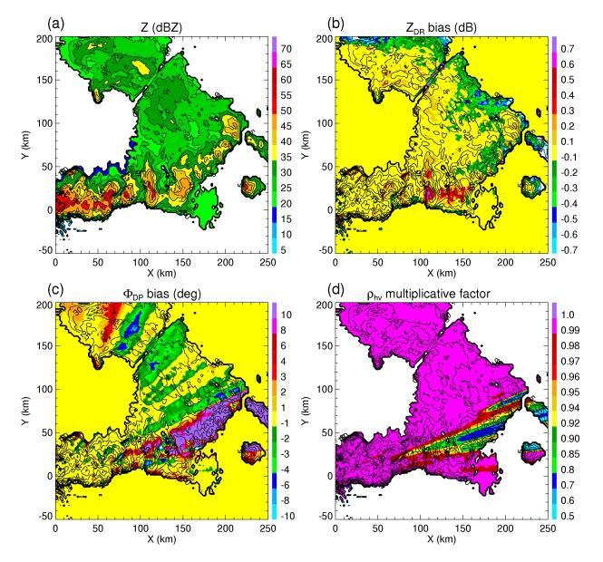
Cross-correlation coefficient is directly affected by the *gradient* of differential phase within the radar resolution volume, not total differential phase which is proportional to path-integrated attenuation
