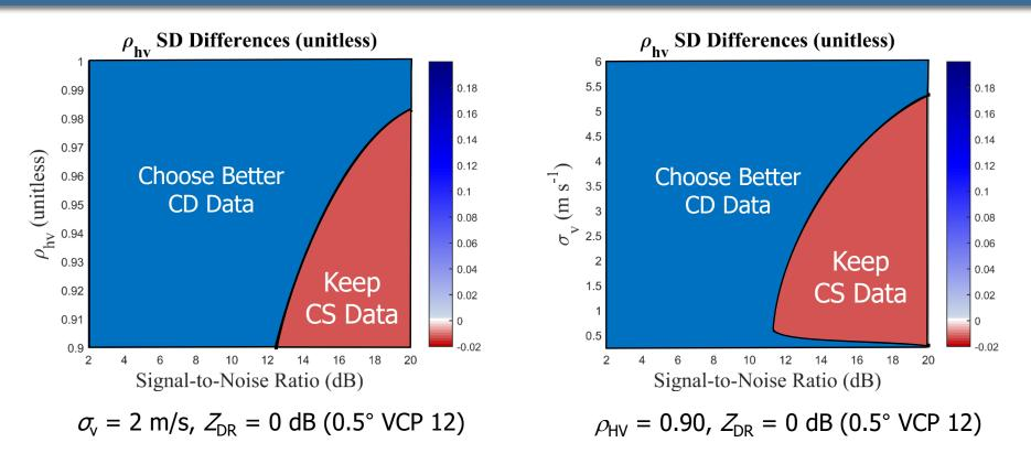
The **HSE** processing **improves** over conventional processing in regions of **low-to-medium SNR** (~0-10 dB) **or relatively high**  $\rho_{HV}$  **or wide**  $\sigma_{V}$
