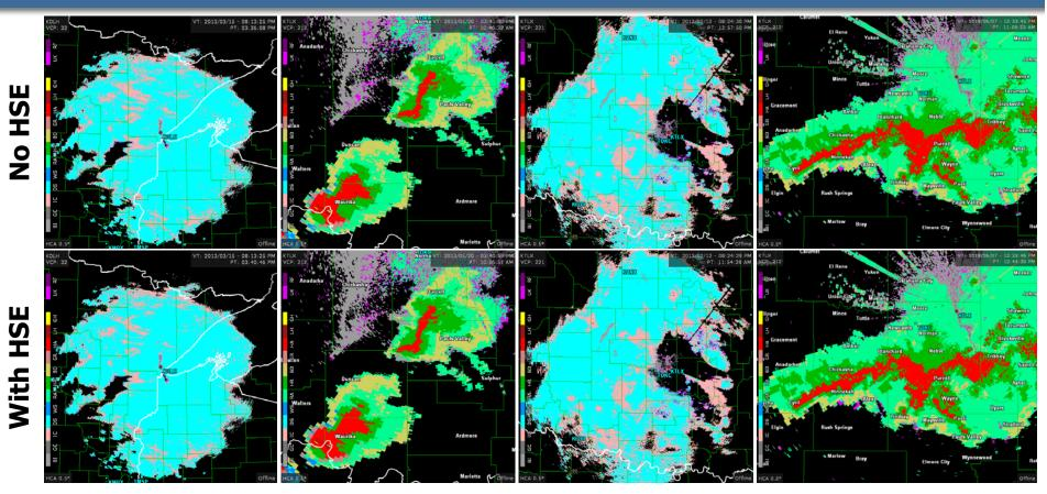
HSE can improve the quality of polarimetric-variable estimates with no harm on the Hydrometeor Classification
