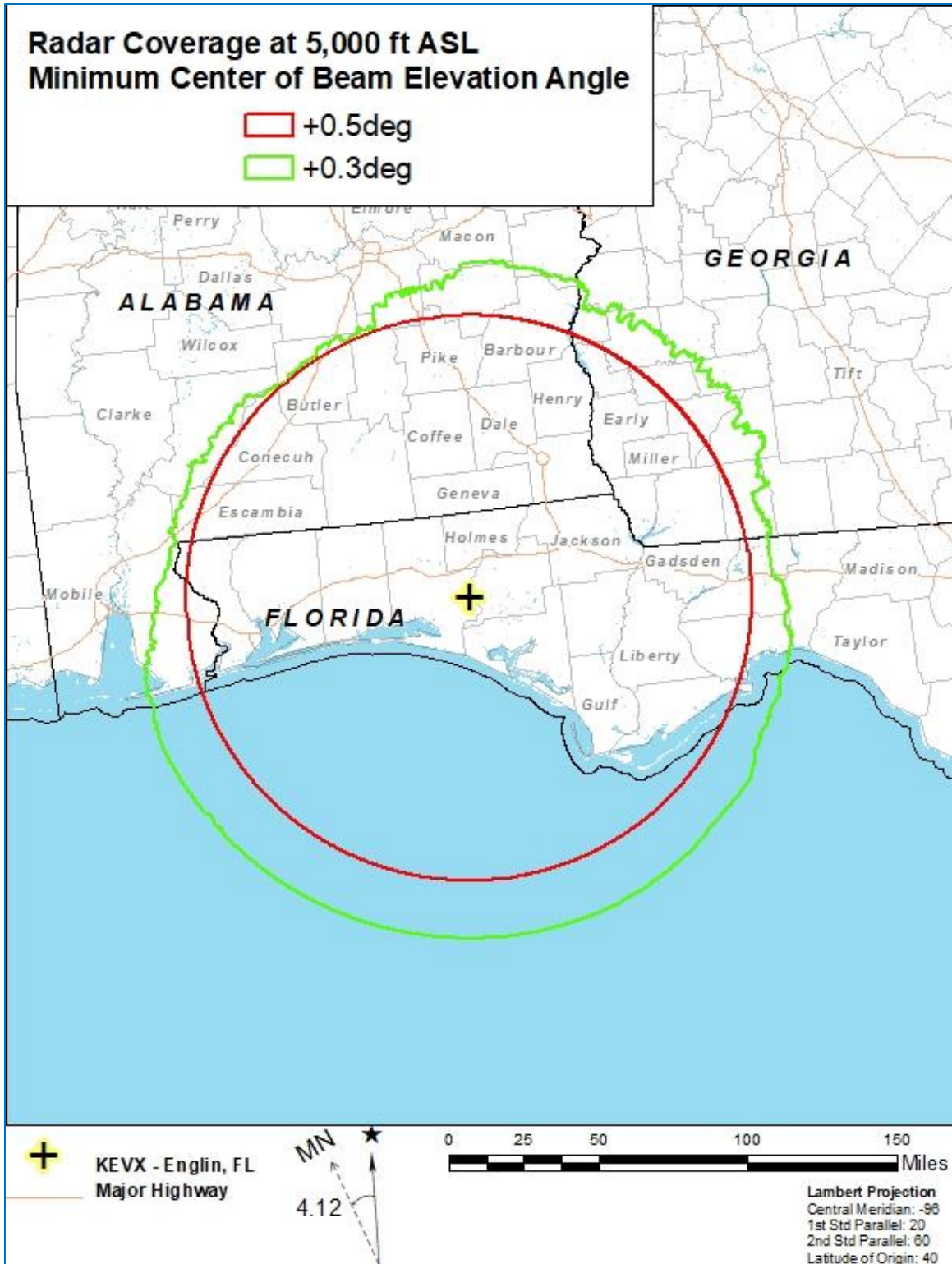
Figure 6: Existing and Proposed KEVX WSR-88D Coverage at 5,000 ft ASL
