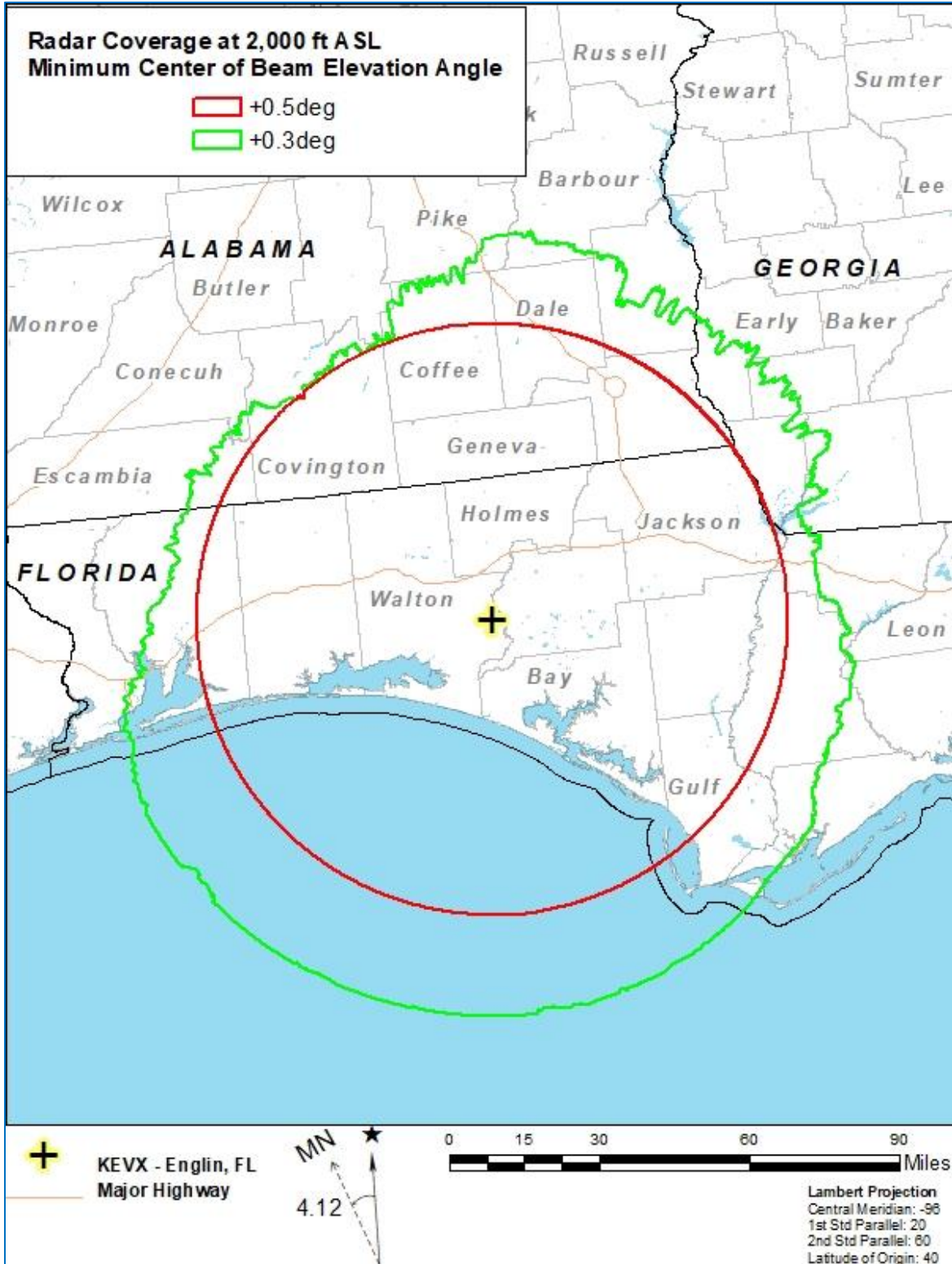
Figure 5: Existing and Proposed KEVX WSR-88D Coverage at 2,000 ft ASL
