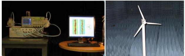
Fig. 8. Model wind turbine (right) and 10 GHz dual-polarized scatterometer (left) in the ARRC Lab at the University of Oklahoma. (Courtesy of the OU ARRC)
