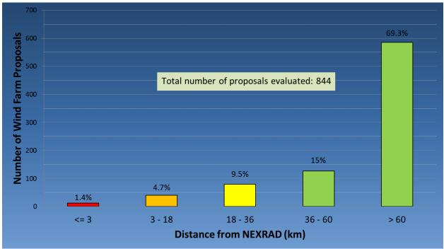
Fig. 5. Number of wind farm proposals as function of distance from a NEXRAD radar.
