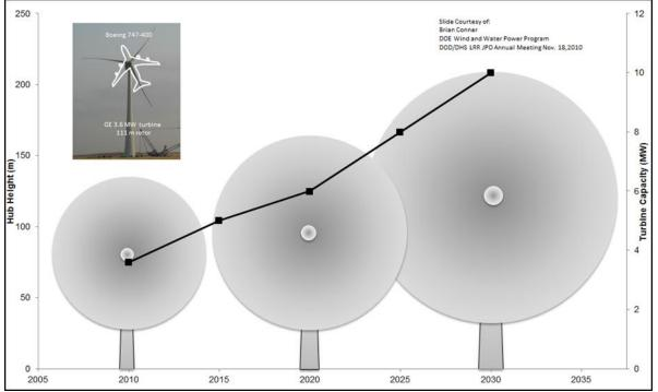
**Fig. 2.** U.S. Department of Energy projected increases in wind turbine height (top dead center) and turbine capacity (black line) from 2010 to 2030. The upper-left depiction of an airplane outline over the hub of a turbine represents the radar cross section a turbine can have, approximately the same as a 747 airliner.
