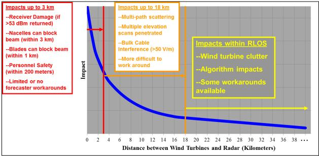
Fig. 4. Inventory of estimated impacts of wind farms on NEXRAD radars relative to the separation distance.
